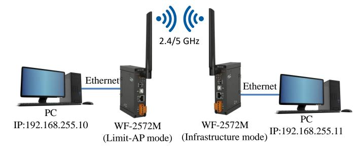
Figure 6. Test Architecture of Limit-AP
