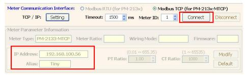
vii. When the system is trying to connect with the power meter, the status information will show "Try connecting" message.
