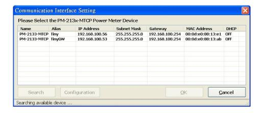
iv. Select the power meter which you want to modify parameters from the meter list, then click "Configuration" button to setup the meter parameters. After complete all setting, click "OK", and return to the meter list windows.
