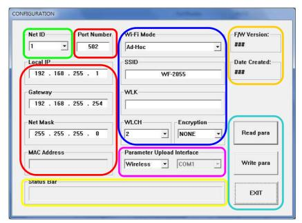
Figure 3-11: Basic Parameter Setting Interface
