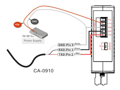
Figure 2-5: Power and Serial port wire connection
