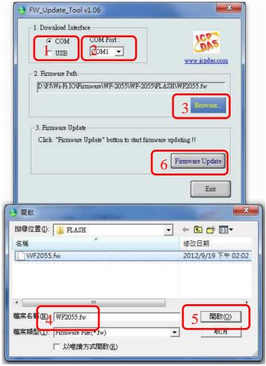
Figure 2-10: WF-2055 firmware update process
