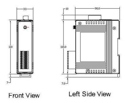
Figure 2-3: Front / Left Side dimension of the WF-2000
