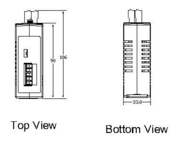
Figure 2-4: Top / Bottom dimension of the WF-2000
