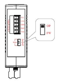
Figure 2-11: OP Position of Dip-Switch
