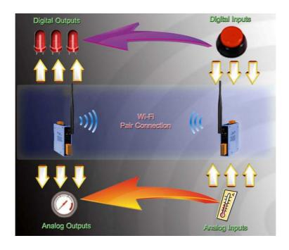
Figure 4-2: Pair connection application architecture
