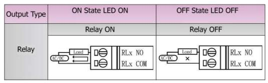
Figure 2-11: DO wire connection
