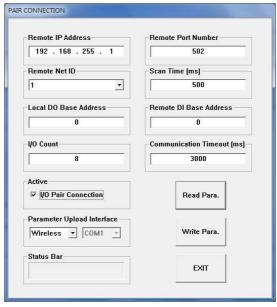
Figure 4-17: Pair connection setting interface
