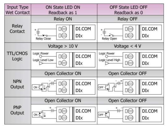
Figure 2-7: WF-2055 DI Wet contact wire connection
