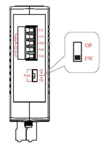
Figure 2-7: FW Position of Dip-Switch
