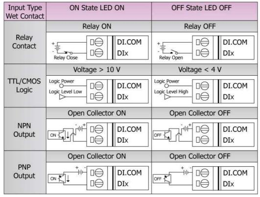
Figure 2-10: DI Wet contact wire connection
