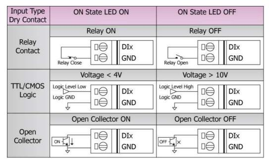
Figure 2-9: DI Dry contact wire connection
