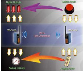
Figure 1-1: I/O Pair Connection of the WF-2000
