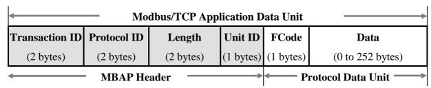
Figure 5-1: Modbus/TCP Application Data Unit
