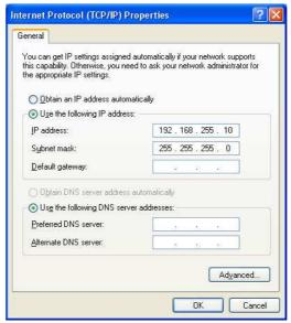
Figure 4-7: IP address setting interface
