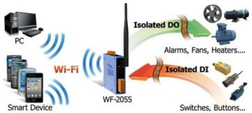
Figure 4-1: WF-2055 + PC application architecture
