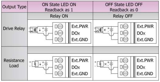
Figure 2-8: WF-2055 DO wire connection
