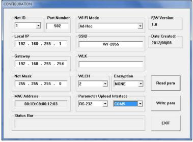
Figure 4-3: Connection Configuration
