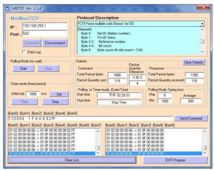
Figure 4-12: DO output control interface
