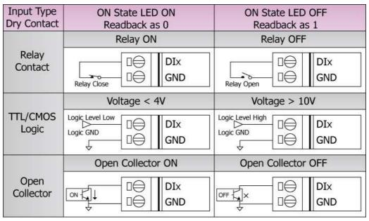
Figure 2-6: WF-2055 DI Dry contact wire connection
