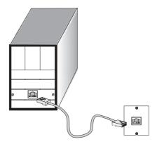
**Step 2.** If the device is a network card and the switch is in the wiring closet, attach the other end of the cable segment to a modular wall outlet that is connected to the wiring closet. (See the section "Network Wiring Connections.") Otherwise, attach the other end to an available port on the switch.
