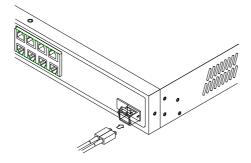
**Step4.** As a connection is made, check the Link LED on the switch corresponding to the port to be sure that the connection is valid.
