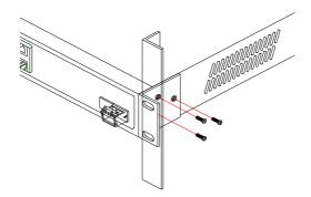
**Step2.** Mount the device in the rack (Via Optional Rack-Mount kit), using four rack-mounting screws (not provided). Be sure to secure the lower rack-mounting screws first to prevent the brackets being bent by the weight of the switch.
