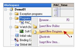
2. Fill in a program name in the "Name" field and enter a simple note in the "Description" field, and then select the "LD – Ladder Diagram" as the programming language and click the "OK" button.
