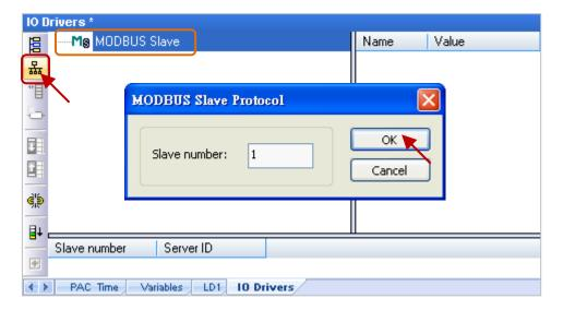
4. Click the "Insert Slave/Data Block" button on the left side to open the "MODBUS Slave Request" window.
