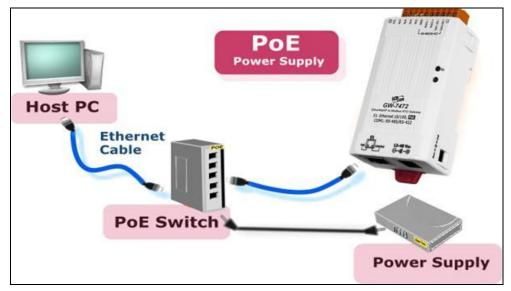
Figure 3.5 GW-7473 with PoE switch power supply
