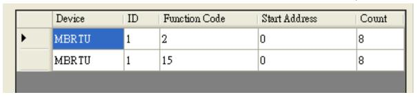
Figure 5.5 Modbus request command
