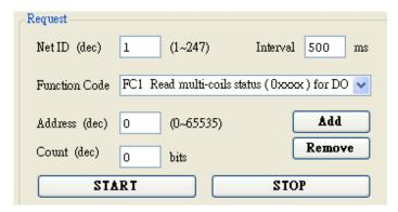
Figure 5.4 Modbus request command
