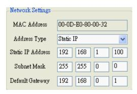
The <u>Address Type</u>, <u>Static IP Address</u>, <u>Subnet Mask</u> and <u>Default Gateway</u> items are the most important network configuration and should always match the LAN definition of your PC. Or, the connection between the GW-7472 and your PC may have problem. Contact your network administrator to obtain a proper network configuration for the GW-7472.
