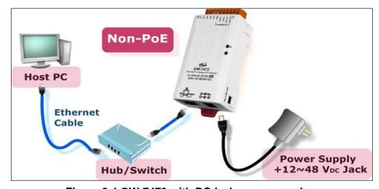
Figure 3.4 GW-7473 with DC jack power supply
