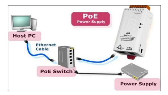
Figure 3.2 GW-7472 with PoE switch power supply
