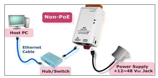
Figure 3.1 GW-7472 with DC jack power supply
