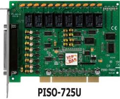
Universal PCI, 8-ch Relay Output and 8-ch Isolated Digital Input Board
