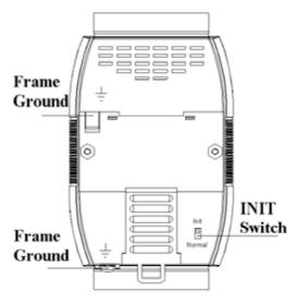
The common features of the I-7013/13D, I-7033/33D, I-7015/15P, M-7015/15P, and M-7033/33D modules are as follows:
