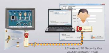
2.Restrict access to some operations in the HMI with the USB security key Assign different access levels for objects or features to enhance security control
