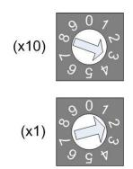
Figure 2-2 Node ID rotary switch
