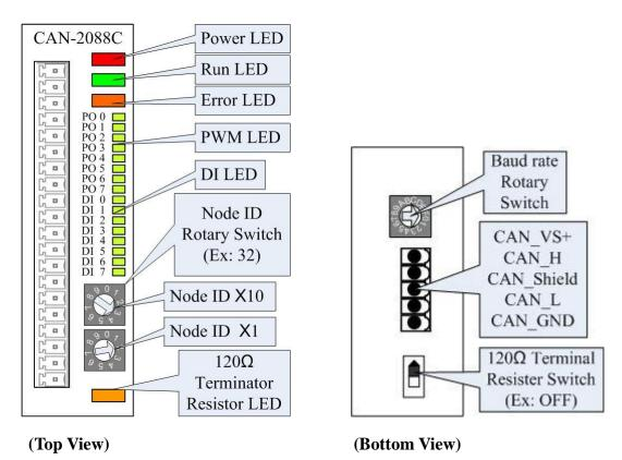
Figure 2-1 CAN-2088C layout of LED, connect, and switch
