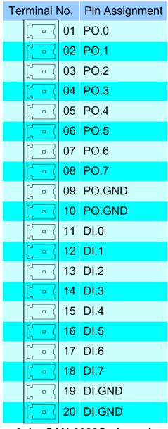
Figure 2-4 CAN-2088C pin assignment
