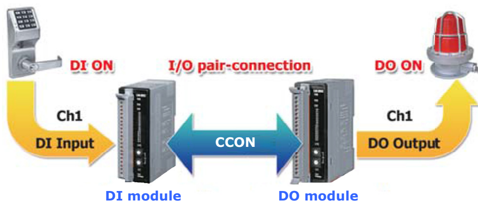
Figure 3-6 I/O pair-connection application
